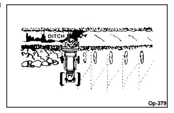
Pile dirt on high side for easier backfilling on a slope.
